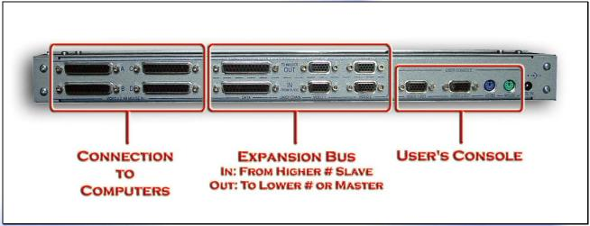
FIGURE 1 MC4-H2 Connector Functions on Rear Panel
